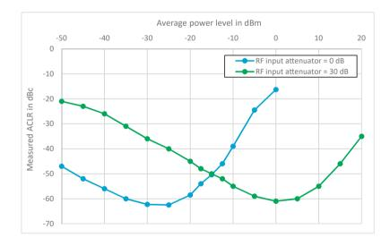
R&S®NRQ6 ALCR performance at 2 GHz over power; EUTRA/LTE 20 MHz (meas., noise correction on).
