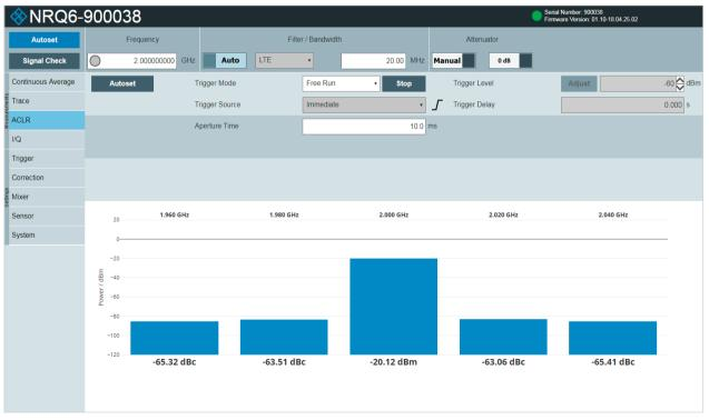
ACLR measurement on a 3.84 MHz 3GPP signal.
