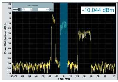
Single-channel power measurement on an MSR signal.
