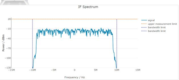
Signal check for a 20 MHz LTE signal.
